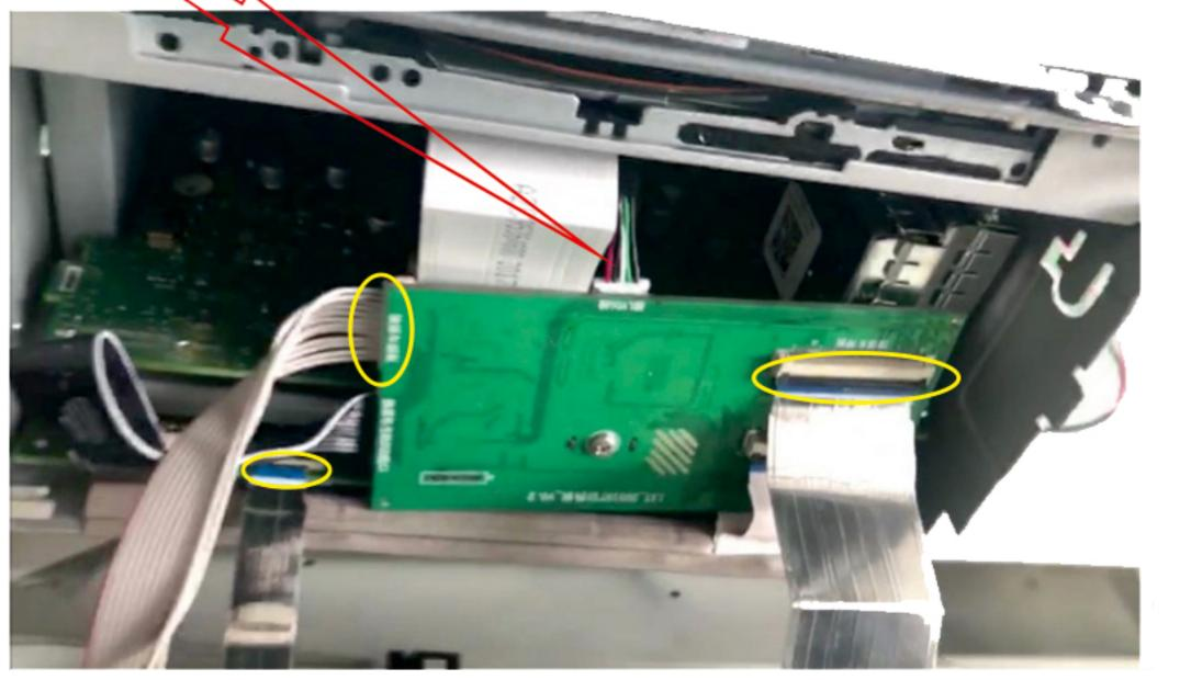
3:Finally restore three factory wires. 50P FFC and 12P wiring into new PCB and SD card wire. Restore panel and screws.
