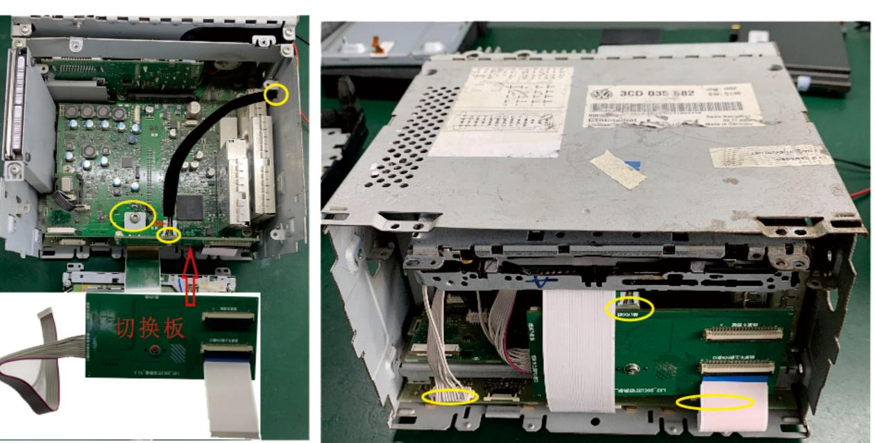
2:Take out PCB from package and install it in the slot, secure with a screw. Insert 50P FFC and 12P wiring into factory slots. Plug LVDS wire and pay attention to headunit entry location. Make sure all wiring are flat to avoid circuit shorting. Restore panel. Result is the picture on the right.
