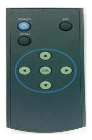
\*FACTORY MODE (Interface setting for installer) : Operated by pressing  $\blacktriangle \rightarrow \lor \rightarrow \land \rightarrow MENU$  button or press  $\blacktriangleleft$  more than 5seconds long on the remote control.
