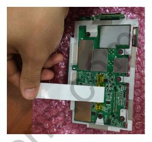
1) Tape up the FFC cable connected to the command and turn over the FFC cable as above..
