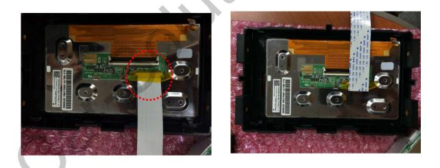
2 Tape up the FFC cable connected to the LCD and turn over the FFC cable as above.
